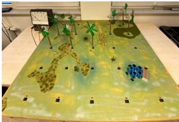
Figure 2-44 – Model of an energy grid with wind turbines, storage units and consumer LED's
